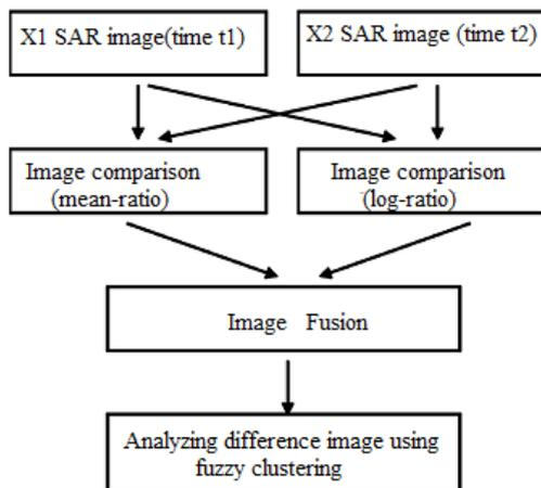
Fig. 1. Flowchart of the change detection approach.
